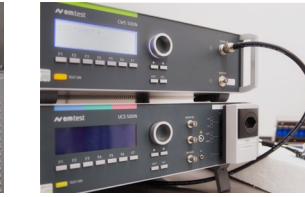
Generators for Surge and Burst
