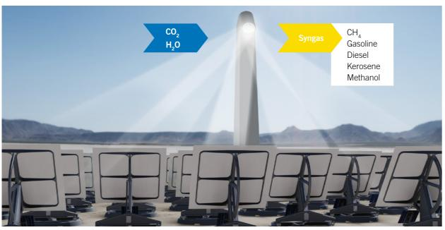
System with solar tower, heliostats and receiver in focus
